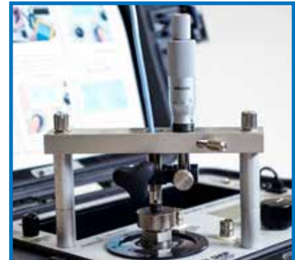
PROXIMITY OPTION 9100-PPA01 fixture is used to check the static and dynamic output of an eddy current proximity probe.
