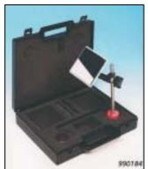
The Type 8329/8335 LDV has two mounting points, at the bottom and side of the sensor unit, each having a <sup>1</sup>/<sub>4</sub>" hole with Whitworth thread, a widespread standard used for camera tripods. Type 8329/8335 can be mounted on the Brüel & Kjær Tripod UA 0989.
